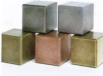
▲ Cubes of different metals have different densities.
